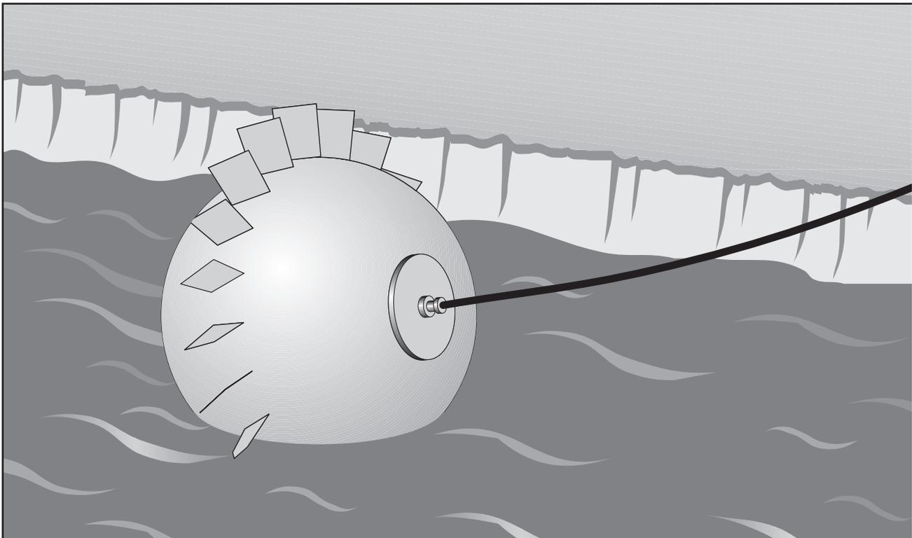
The PHEPP makes electrical energy from movement energy in the same way as a bicycle dynamo (see Figure 2). The movement of the water pushes against blades on the outside of the PHEPP and turns it while the inside stays still held by a weight.
